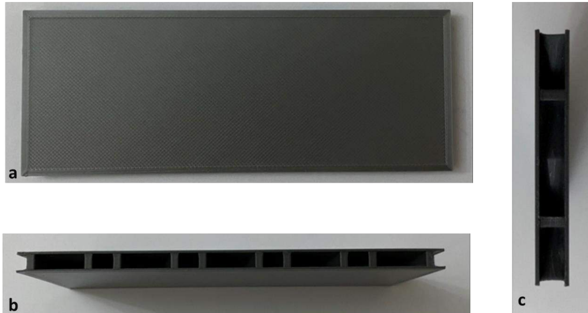
Figure 2.5: Sandwich Panel After Adhesion; a) Front view, b) Top view c) Side view
